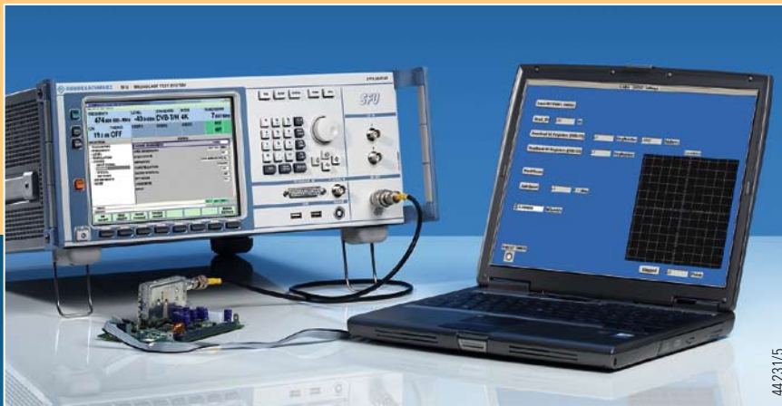
FIG 3 With its capabilities to modify and impair signals and to simulate interference, the R&S®SFU simulates rough ambient conditions in the lab under which chips and tuners can be tested to the limits of their functionality.
